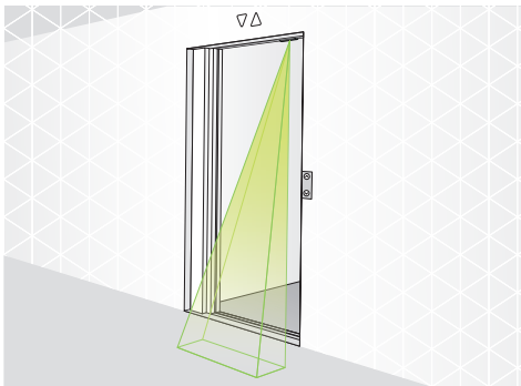
Figure 1: IMS 100 Pro - corner-mounted for side-opening doors
